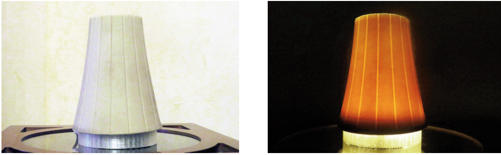
Figg. 16, 17 - Experimentation with a composite lamp obtained with a silicone mould, with a natural light effect and backlit (credits: F. Valente, 2018).
