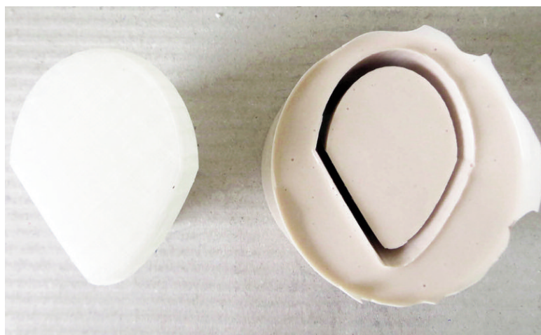
Fig. 14, 15 - Silicone mould and composite samples obtained (credits: F. Valente, 2018).
